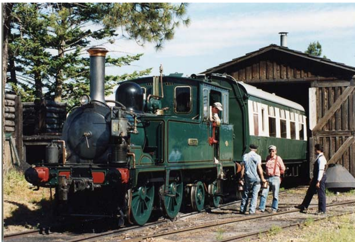
Dunrobin at Fort Steele, Canada. This 0-4-4T locomotive was built by Sharp Stewart in 1895 for the Duke of Sutherland to haul his private train at Dunrobin Castle, Scotland and did so until c1920. After a period on display the locomotive and carriage were exported to Canada in 1965 where it remained in operation until 2005. After negotiations the locomotive and its private saloon was bought by Beamish Museum, Co. Durham in December 2010 and returned to England in May 2011.
